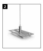
Screw the rail sliders to the cable holder with the M6 hexagon nut and the serrated lock washer. Push the wire cable through the cable holder and adjust the running rails to working height. Then raise the ceiling element to working height and place it on mounting blocks if necessary.
